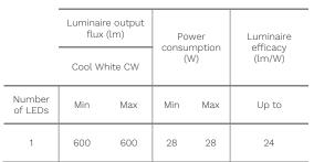
Tolerance on LED flux is  $\pm$  7% and on total luminaire power  $\pm$  5 %
