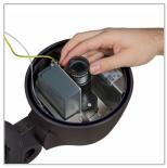
As with all VALINTAs, the GOBO model features tilt and swivel adjustment, to ensure that the projected image is sharp and undistorted by allowing the best projection angle to be selected. The convenience of the easy open mechanism and rotating zoom lens ensures quick focus adjustments on site. A removable magnetic holder makes it easy to change GOBO images. And with optional DMX control, light intensity can be fine-tuned, making
