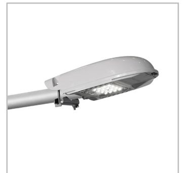
Precise on-site adjustment. The inclination angle can be set from -15° to +5° for side-entry mounting, and from -10° to +10° with the post-top adaptor.
